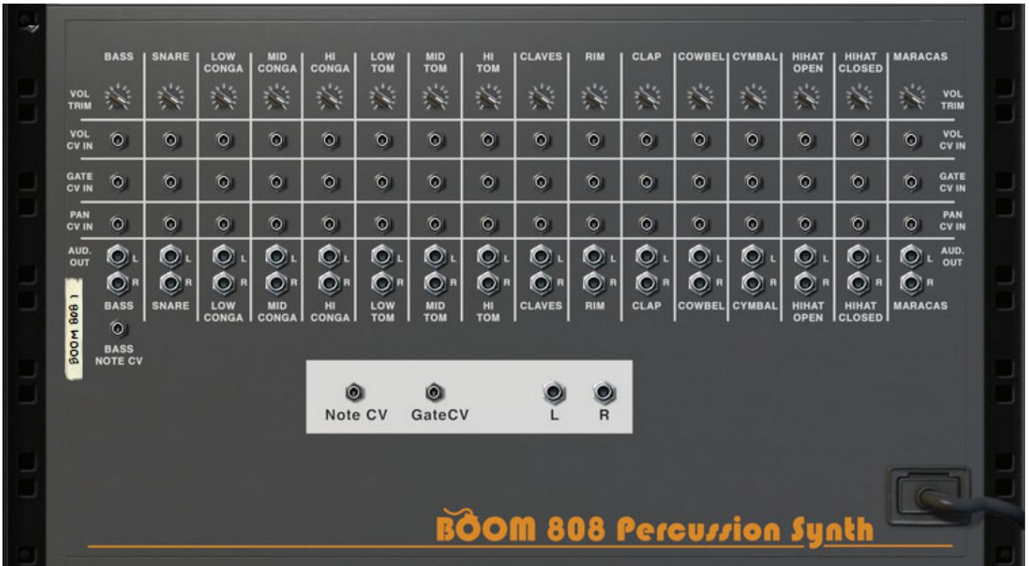
BOOM 808 has a variety of audio and CV connections to enable many creative options. In addition to main outputs and CV connections (shown by a white box), each instrument has its own individual connections available.
